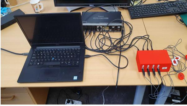
Fig. 2: Complete acquisition system. The red box is the connection box for powering the microphones. The black box is the sound card for digitizing the sound signal and a laptop for saving the data.
